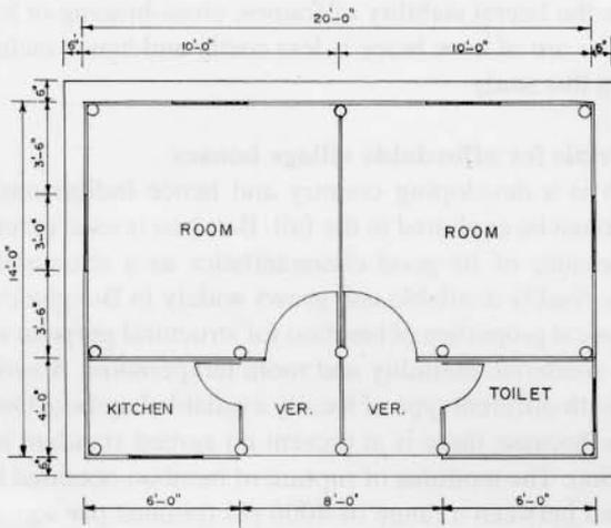
Fig. 2 : Plan of Proposed Low Cost House
