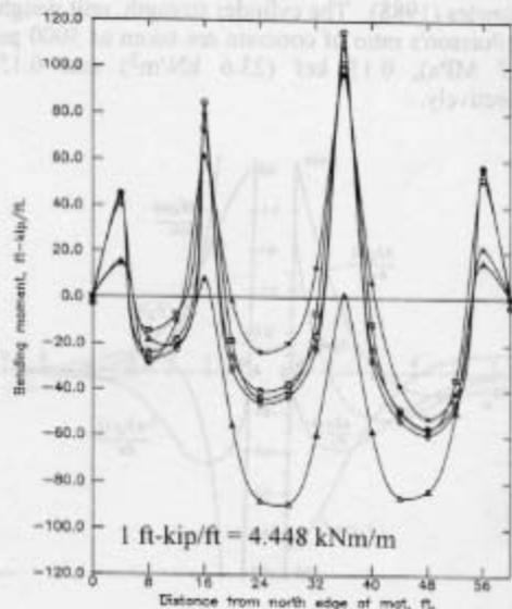
Fig. 6 Comparison of moments along column line 3
