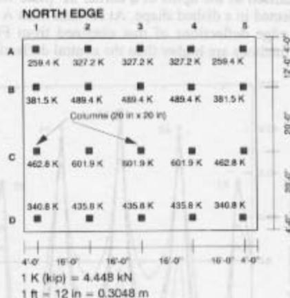
Fig. 2 Mat dimensions with column loads
